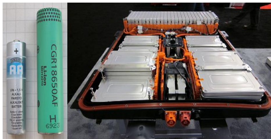
Figure 2. 4: Alkaline AA battery cell, Tesla lithium-ion battery cell, and Nissan battery modules and pack. [27].
