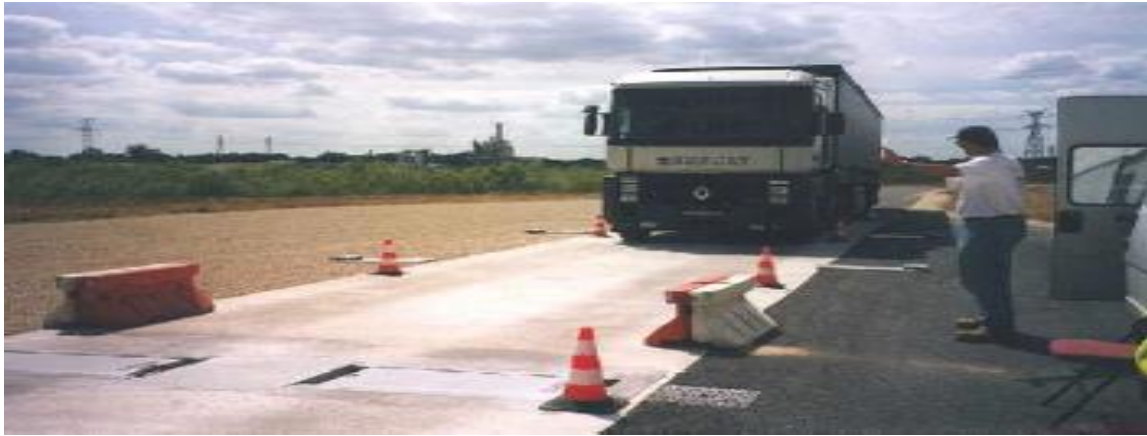
Fig. 3 weight in motion (WIM) overload vehicle detection system {Source:Low Speed WIM using load cell wheel scales in a concrete platform (Châlon s/Saône, France).}
