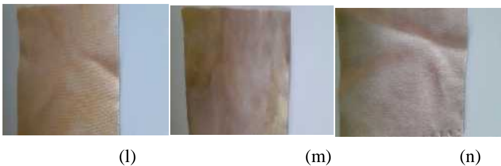
Figure-24 : (h) Direct dyeing(without mordant) of nylon fiber.(i) Pre mordant( \text{FeSO}_4 ) dyeing of nylon fiber.(j) Simultaneous mordant( \text{FeSO}_4 ) dyeing of nylon fiber.(k) Post mordant( \text{FeSO}_4 ) dyeing of nylon fiber.(l) Pre mordant( \text{CuSO}_4 ) dyeing of nylon fiber.(m) Simultaneous mordant( \text{CuSO}_4 ) dyeing of nylon fiber.(n) Post mordant ( \text{CuSO}_4 ) dyeing nylon fiber.
