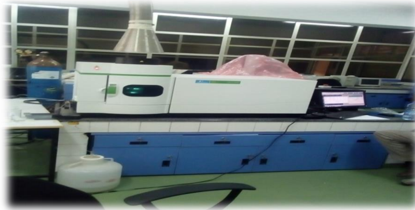
Figure: 3.3 shows ICP-OES used for the determination of heavy metals (Zn, Cu, Cd &Pb) from digested rice samples
