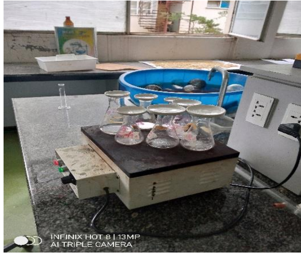
Appendence 1: Digestion of samples to determine metal on hot plate
