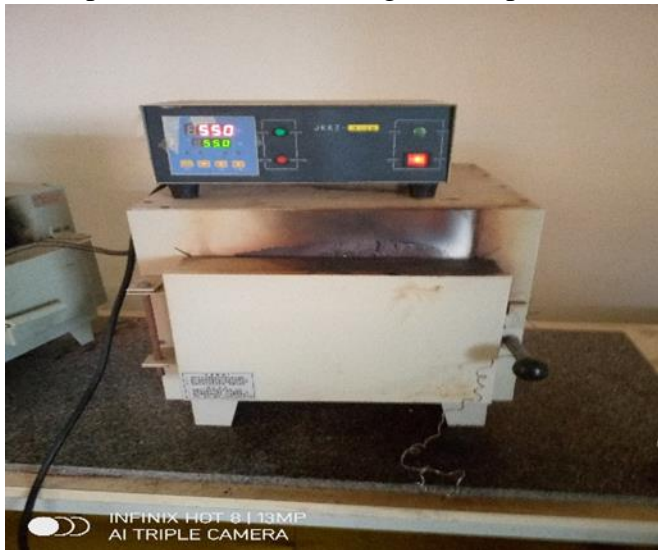
Appendence 2: Sample in muffle furnace (ignite samples)
