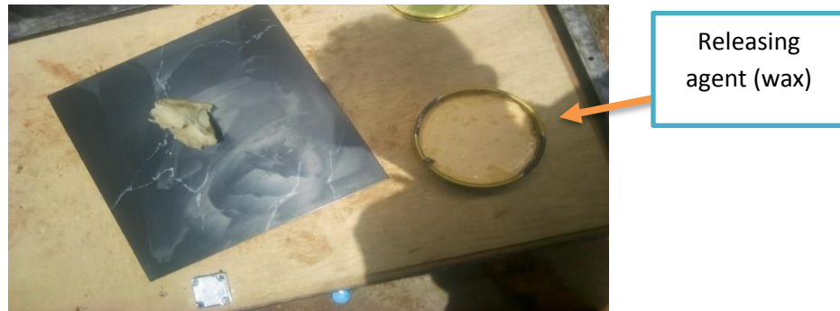
Figure 3. 30 Painting of releasing agent to the mold
