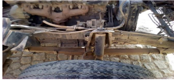
Figure 3.15, Mounting of steel leaf spring [Observation]
