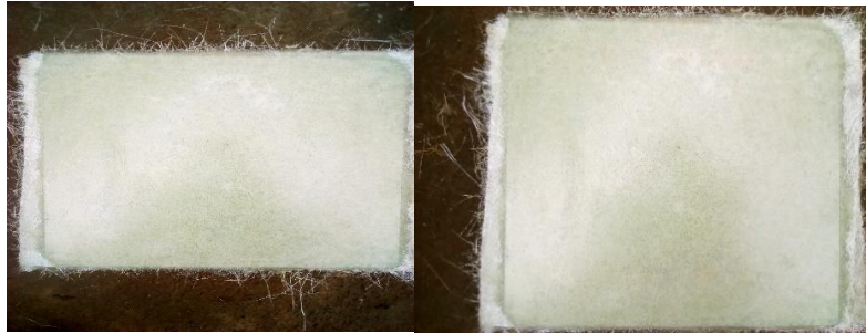
Figure 3. 32 Untrimmed composite material
