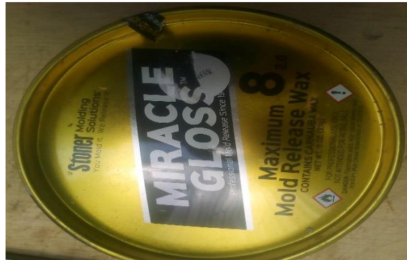
Figure 3. 26 Releasing agent of molds
