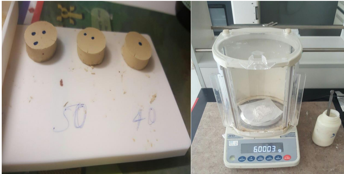
FigureA5. 5 The sample after sintering and the powder weigh up in electrical balance
