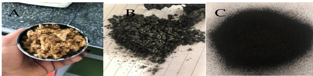
Figure 3-1: processes of bamboo activated carbon preparation
