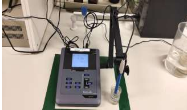
Figure 3.6 PH meter: model no. PH 7310 & PH 7310 P
