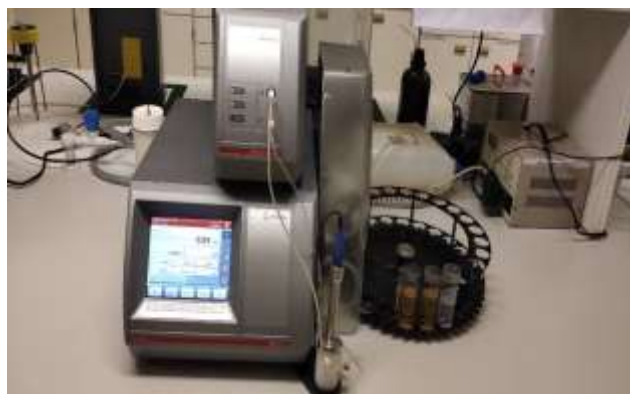
Figure 3.5 Anton Paar alcoholizer: Model no. 4500
