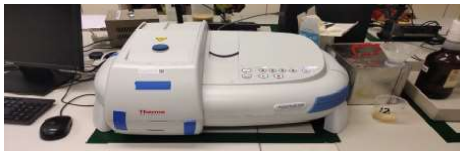
Figure 3.7 UV-VIS spectrophotometer: Model no.840-210600
