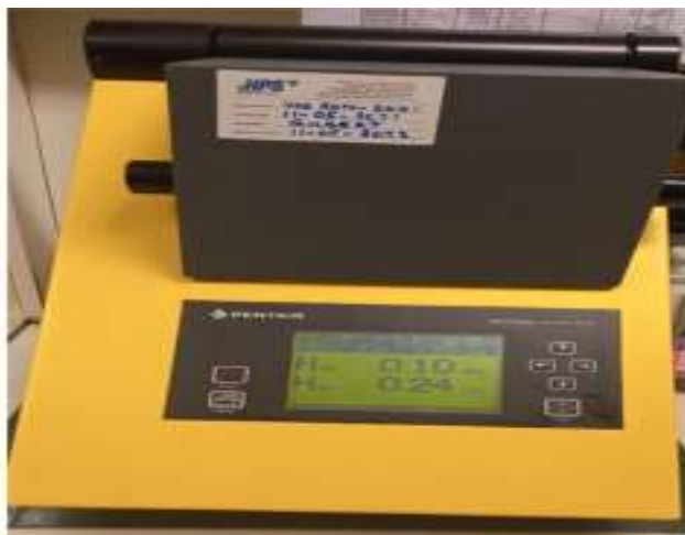
Figure 3.8 Turbidity meters: Model no. Haffmans Vos Rota 90/25
